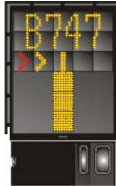
The vertical yellow arrow shows position in relation to the centre line. This indicator gives correct position and azimuth guidance.
